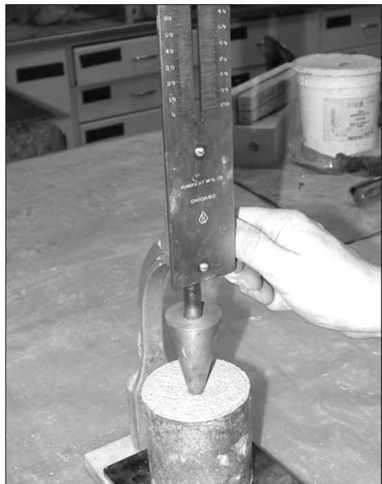
Figure 3. The Vicat cone is dropped into a cylinder of mortar; the depth of penetration provides an indication of the mortar consistency.
